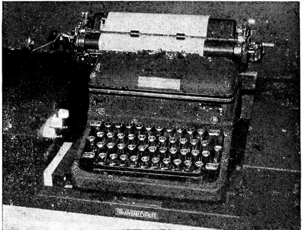
Standard typewriter adapted for feeding teleprinter circuits. Light source unit is at right, while phototubes, thyatrons, and associated relays are in housing at left, with pilot lamps and control switches conveniently near the typewriter shift key
